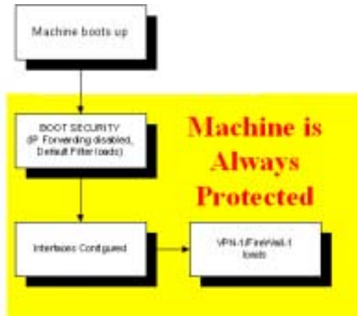
FIGURE A-1 How a Default Filter Protects the VPN-1/FireWall-1 Gateway computer
